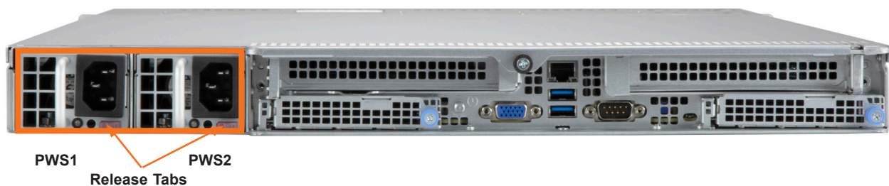
Figure 3-11. Replacing the Power Supply
