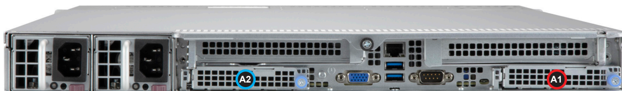
Figure 3-12. AIOM Chassis Slots
